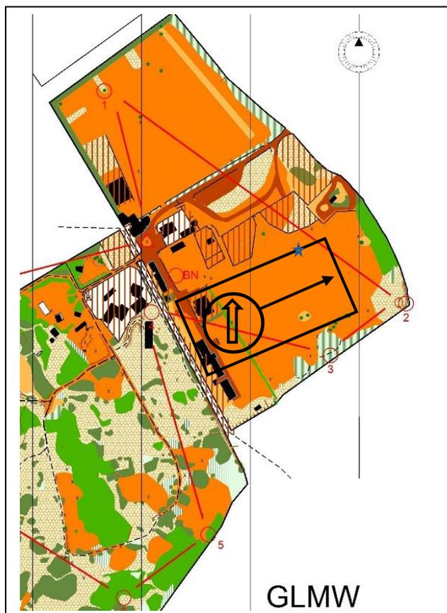
Let's say we're going to work out what the bearing of the tree in the middle of the field is. With the edge lined up with where you are and the tree, turn the dial until the lines and arrow in the dial are in line with the magnetic north lines on the map.
